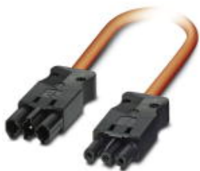
Power cable, 3-position, PVC, orange RAL 2004, Plug straight, black, on Socket straight, black, cable length: 1 m
