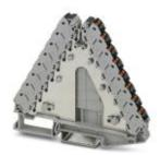
Potential distributors, nom. voltage: 250 V, nominal current: 17.5 A, cross section: 0.14 mm² - 2.5 mm², AWG: 14 - 26, connection method: Push-in connection, number of positions: 2, number of connections: 32, width: 8.3 mm, length: 100 mm, color: gray, color of connection elements: black, mounting: NS 35/7,5, NS 35/15
