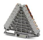
Marshalling panel, nom. voltage: 250 V, nominal current: 8 A, cross section: 0.14 mm² - 2.5 mm², AWG: 14 - 26, connection method: Push-in connection, number of positions: 2, number of connections: 32, width: 8.3 mm, length: 100 mm, color: gray, color of connection elements: red, white, mounting: NS 35/7,5, NS 35/15
