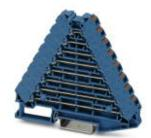
Marshalling panel, nom. voltage: 250 V, nominal current: 8 A, cross section: 0.14 mm² - 2.5 mm², AWG: 14 - 26, connection method: Push-in connection, number of positions: 2, number of connections: 32, width: 8.3 mm, length: 100 mm, color: blue, color of connection elements: blue, mounting: NS 35/7,5, NS 35/15
