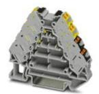
Potential distributors, nom. voltage: 250 V, nominal current: 17.5 A, cross section: 0.14 mm² - 2.5 mm², AWG: 14 - 26, connection method: Push-in connection, number of positions: 2, number of connections: 16, width: 8.3 mm, length: 64 mm, color: gray, color of connection elements: yellow, black, mounting: NS 35/7,5, NS 35/15
