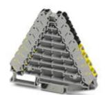
Potential distributors, without actuation lever, nom. voltage: 250 V, nominal current: 17.5 A, cross section: 0.14 mm² - 2.5 mm², AWG: 14 - 26, connection method: Push-in connection, number of positions: 2, number of connections: 32, width: 8.3 mm, length: 100 mm, color: gray, color of connection elements: black, yellow, mounting: NS 35/7,5, NS 35/15
