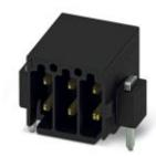
PCB headers, nominal current: 6 A, rated voltage (III/2): 160 V, number of positions: 3, pitch: 2.54 mm, color: black, contact surface: Gold, mounting: SMD soldering
