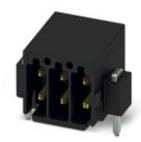
PCB headers, nominal current: 6 A, rated voltage (III/2): 160 V, number of positions: 2, pitch: 2.54 mm, color: black, contact surface: Gold, mounting: SMD soldering
