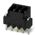
PCB headers, nominal current: 6 A, rated voltage (III/2): 160 V, number of positions: 2, pitch: 2.54 mm, color: black, contact surface: Gold, mounting: THR soldering
