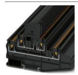
Fuse modular terminal block, fuse type: Glass / ceramics / ..., connection method: Push-in connection, cross section:  $0.2 \text{ mm}^2$ -  $6 \text{ mm}^2$ , AWG: 24 - 10, nominal current: 28 A, nom. voltage: 500 V, width: 6.2 mm, fuse type:  $6 \text{ J} \times 20$ , mounting type: NS 35/7,5, NS 35/15, color: black
