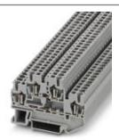
Component terminal block, with integrated diode 1N 5408K, nom. voltage: 500 V, nominal current: 1.5 A, connection method: Spring-cage connection, cross section:  $0.08 \text{ mm}^2$  -  $4 \text{ mm}^2$ , AWG: 28 - 12, length: 67.5 mm, width: 5.2 mm, color: gray, mounting: NS 35/7.5, NS 35/15, nom. voltage: 500 V
