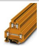
Feed-through terminal block, connection method: Screw connection, cross section: 0.2 mm² - 4 mm², AWG: 24 - 12, width: 6.2 mm, color: orange, mounting type: NS 35/7,5, NS 35/15, NS 32
