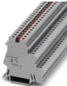
Sensor/actuator terminal block, connection method: Screw connection, cross section: 0.2 mm 2 - 4 mm 2 , AWG: 24 - 12, width: 6.2 mm, color: gray, mounting type: NS 35/7,5, NS 35/15
