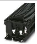
Fuse modular terminal block, fuse type: Glass / ceramics / ..., connection method: Screw connection, cross section:  $0.2 \text{ mm}^2$ - 4 mm², AWG: 24 - 12, nominal current: 6.3 A, nom. voltage: 800 V, width: 8.2 mm, fuse type: G /  $5 \times 20 / 5 \times 25 / 5 \times 30$ , mounting type: NS 35/7,5, NS 35/15, NS 32, color: yellow
