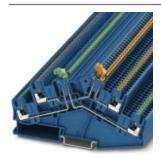
Knife disconnect terminal block, Double level with angled contour and two disconnect knives, nom. voltage: 400 V, nominal current: 16 A, connection method: Push-in connection, cross section: 0.14 mm² - 4 mm², AWG: 26 - 12, length: 127.5 mm, width: 5.2 mm, color: blue, mounting: NS 35/7,5, NS 35/15, nom. voltage: 400 V
