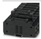
Fuse modular terminal block, fuse type: Glass / ceramics / ..., connection method: Screw connection, cross section:  $0.75~\text{mm}^2$ -  $25~\text{mm}^2$ , AWG: 18 - 4, nominal current: 32~A, nom. voltage: 1500~V, width: 23~mm, fuse type: gG / gPV / 10.3~x 85, mounting type: NS 35/7,5, NS 35/15, color: black
