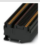
Fuse modular terminal block, fuse type: Flat, connection method: Push-in connection, cross section: 0.5 mm²-10 mm², AWG: 20 - 8, nominal current: 25 A, nom. voltage: 24 V, width: 8.2 mm, fuse type: C, mounting type: NS 35/7,5, NS 35/15, color: black
