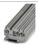
Component terminal block, nom. voltage: 800 V, nominal current: 0.5 A, connection method: Spring-cage connection, number of connections: 3, cross section:  $0.08 \text{ mm}^2$  -  $4 \text{ mm}^2$ , AWG: 28 - 12, width: 5.2 mm, color: gray, mounting type: NS 35/7.5, NS 35/15
