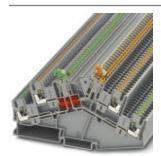
Knife disconnect terminal block, Double level with angled contour and two disconnect knives, nom. voltage: 400 V, nominal current: 16 A, connection method: Push-in connection, cross section: 0.14 mm² - 4 mm², AWG: 26 - 12, length: 127.5 mm, width: 5.2 mm, color: gray, mounting: NS 35/7,5, NS 35/15, nom. voltage: 400 V
