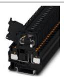
Fuse modular terminal block, fuse type: Glass / ceramics / ..., connection method: Push-in connection, cross section:  $0.2 \text{ mm}^2$ -  $6 \text{ mm}^2$ , AWG: 24 - 10, nominal current: 6.3 A, nom. voltage: 250 V, width: 6.2 mm, fuse type: G /  $5 \times 20$ , mounting type: NS 35/7.5, NS 35/15, color: blue
