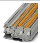
Knife disconnect terminal block, nom. voltage: 400 V, nominal current: 20 A, connection method: Quick connection, cross section: 0.5 mm² - 2.5 mm², AWG: 20 - 14, length: 79.3 mm, width: 6.2 mm, color: gray, mounting: NS 35/7,5, NS 35/15, nom. voltage: 400 V
