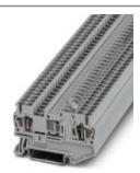
Knife disconnect terminal block, Disconnect knife in gray, nom. voltage: 400 V, nominal current: 20 A, connection method: Spring-cage connection, cross section: 0.08 mm² - 4 mm², AWG: 28 - 12, length: 60.5 mm, width: 5.2 mm, color: gray, mounting: NS 35/7,5, NS 35/15, nom. voltage: 400 V
