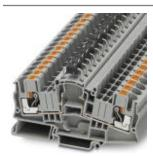
Component terminal block, with integrated P1000Y diode, connection method: Push-in connection, cross section:  $0.5~\text{mm}^2$  -  $10~\text{mm}^2$  , AWG: 20~--10, width: 8.2~mm, color: gray
