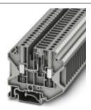
Disconnect terminal block, nom. voltage: 500 V, nominal current: 20 A, connection method: Screw connection with spring support, cross section: 0.2 mm² - 6 mm², AWG: 24 - 10, length: 63.4 mm, width: 6.2 mm, color: gray, mounting: NS 35/7,5, NS 35/15, NS 32, nom. voltage: 500 V
