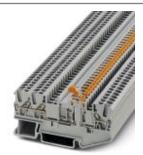
Knife disconnect terminal block, nom. voltage: 400 V, nominal current: 18 A, connection method: Leg spring connection, number of connections: 3, cross section: 0.2 mm² - 4 mm², AWG: 24 - 12, width: 5.2 mm, height: 35.3 mm, color: gray, mounting type: NS 35/7,5, NS 35/15
