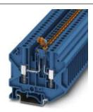
Knife disconnect terminal block, nom. voltage: 500 V, nominal current: 20 A, connection method: Screw connection with spring support, cross section:  $0.2 \text{ mm}^2$  -  $6 \text{ mm}^2$ , AWG: 24 - 10, length: 63.4 mm, width: 6.2 mm, color: blue, mounting: NS 35/7.5, NS 35/15, NS 32, nom. voltage: 500 V
