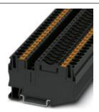
Fuse modular terminal block, fuse type: Flat, connection method: Push-in connection, cross section: 0.5 mm²-10 mm², AWG: 20 - 8, nominal current: 25 A, nom. voltage: 400 V, width: 8.2 mm, fuse type: C, mounting type: NS 35/7,5, NS 35/15, color: black
