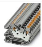
Installation terminal block, Push-in connection, cross section: 0.5 mm² - 16 mm², AWG: 24 - 4, width: 10.2 mm, color: gray, mounting type: NS 35/7,5, NS 35/15
