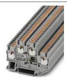
Component terminal block, with integrated 1N4007 diode, nom. voltage: 500 V, nominal current: 20 A, connection method: Push-in connection, number of connections: 4, cross section: 0.14 mm² - 4 mm², AWG: 26 - 12, width: 5.2 mm, color: gray, mounting type: NS 35/7,5, NS 35/15
