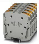
High-current terminal block, nom. voltage: 1000 V AC / 1500 V DC, nominal current: 150 A, connection method: Power-Turn connection, number of connections: 2, cross section: 10 mm² - 70 mm², AWG: 8 - 2/0, width: 20 mm, color: gray, mounting type: NS 35/15
