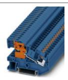
N disconnect terminal block, Push-in connection, cross section:  $0.2 \text{ mm}^2$  -  $6 \text{ mm}^2$ , AWG: 24 - 10, width: 6.2 mm, color: blue, mounting type: NS 35/7.5, NS 35/15
