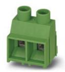
PCB terminal block, nominal current: 32 A, nom. voltage: 1000 V, pitch: 9.52 mm, number of positions: 3, connection method: Screw connection with tension sleeve, mounting: Wave soldering, conductor/PCB connection direction: 0 °, color: green. The article can be aligned to create different nos. of positions!
