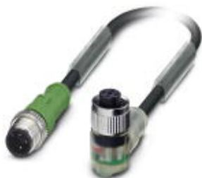
Sensor/actuator cable, 3-position, PUR halogen-free, black-gray RAL 7021, Plug straight M12, A-coded, on Socket angled M12, A-coded, with 2 LEDs, PIN 2+4 bridged, cable length: 5 m
