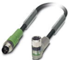
Sensor/actuator cable, 3-position, PUR, black-gray RAL 7021, Plug straight M8, A-coded, on Socket angled M8, A-coded, with 2 LEDs, cable length: 2 m
