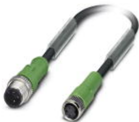
Sensor/actuator cable, 3-position, PUR halogen-free, black-gray RAL 7021, Plug straight M12, A-coded, on Socket straight M8, cable length: 1 m
