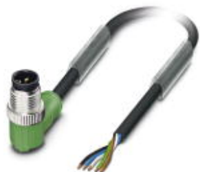
Sensor/actuator cable, 5-position, PVC, black RAL 9005, Plug angled M12, A-coded, on free cable end, cable length: 5 m
