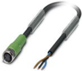
Sensor/actuator cable, 3-position, PVC, black RAL 9005, free cable end, on Socket straight M8, cable length: 3 m
