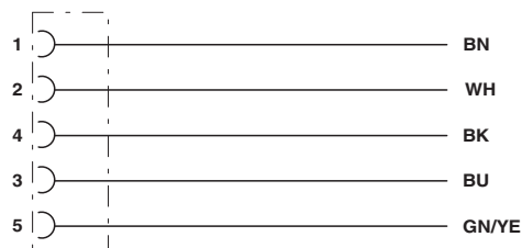
Contact assignment of the M12 sockets
