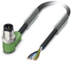
Sensor/actuator cable, 5-position, PVC, black RAL 9005, Plug angled M12, A-coded, on free cable end, cable length: 3 m
