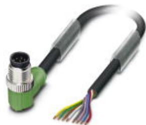
Sensor/actuator cable, 8-position, PVC, black RAL 9005, Plug angled M12, A-coded, on free cable end, cable length: 5 m
