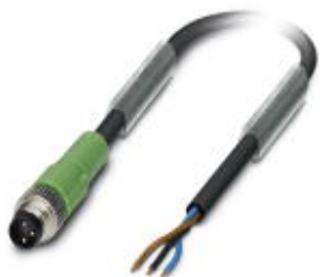
Sensor/actuator cable, 3-position, PVC, black RAL 9005, Plug straight M8, on free cable end, cable length: 3 m
