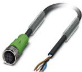
Sensor/actuator cable, 4-position, PVC, black RAL 9005, free cable end, on Socket straight M12, A-coded, cable length: 1.5 m
