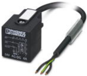
Sensor/actuator cable, 3-position, PVC, black RAL 9005, free cable end, on Valve connector A, with 1 LED, connected with Z diode, cable length: 1 m
