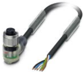
Sensor/actuator cable, 5-position, PVC, black RAL 9005, free cable end, on Socket angled M12, A-coded, with 3 LEDs, cable length: 1.5 m
