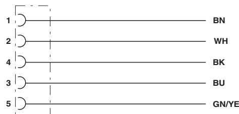
Contact assignment of the M12 sockets
