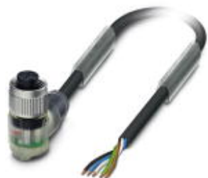
Sensor/actuator cable, 5-position, PVC, black RAL 9005, free cable end, on Socket angled M12, A-coded, with 3 LEDs, cable length: 3 m
