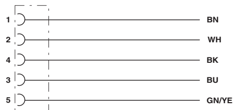
Contact assignment of the M12 sockets
