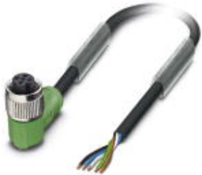
Sensor/actuator cable, 5-position, PVC, black RAL 9005, free cable end, on Socket angled M12, A-coded, cable length: 1.5 m
