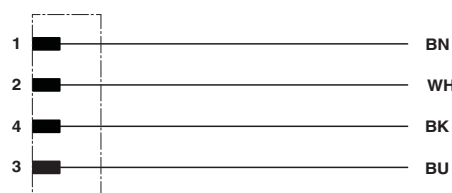
Contact assignment of the M12 plug
