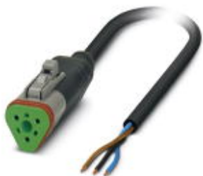
Sensor/actuator cable, 3-position, PUR halogen-free, black-gray RAL 7021, free cable end, on Socket straight DEUTSCH DT06-3S Clip locking, cable length: 1.5 m
