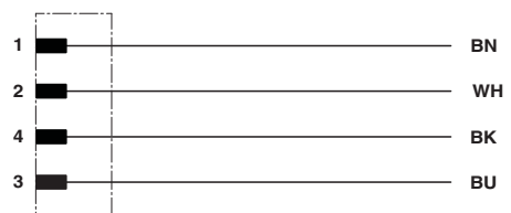
Contact assignment of the M8 plug
